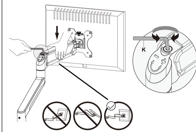
**Note:** Be sure to keep the arm in a horizontal position during adjustment. Or else it would be difficult to adjust the mount or damage the mount.
