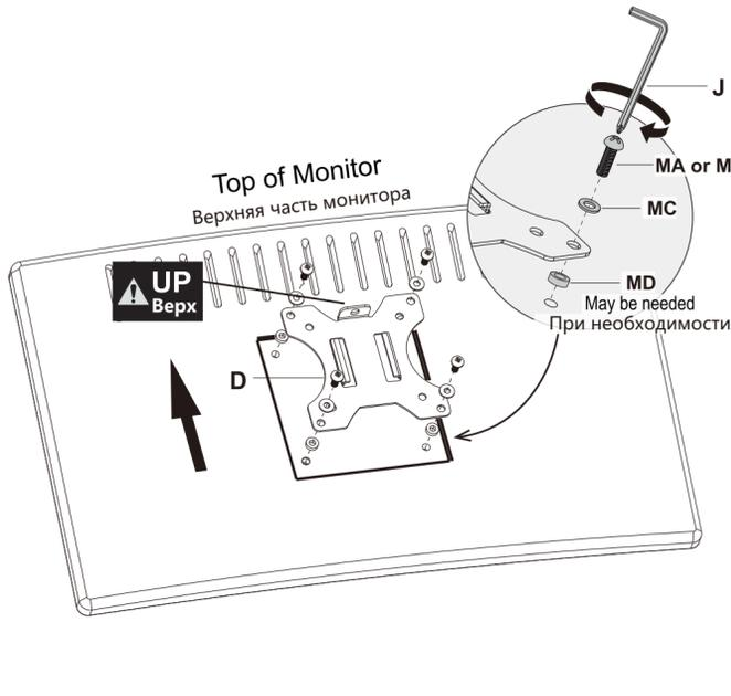
Do not tighten the screws excessively or tighten them by using the Electrodrill, or your monitor might be damaged.
