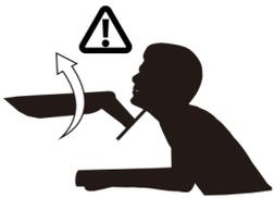
Tension adjustment should be done only after monitor installation
