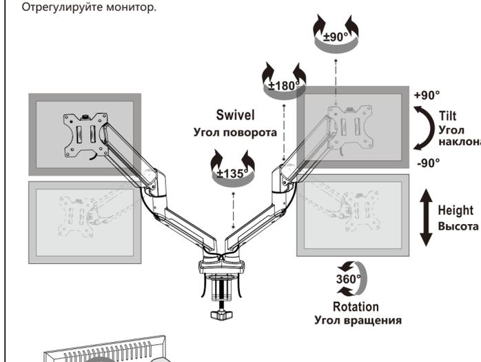
**Note:** To ensure stability, the tightness of the rotating axis has been preset, so it would be kind of difficult to rotate the VESA plate.
